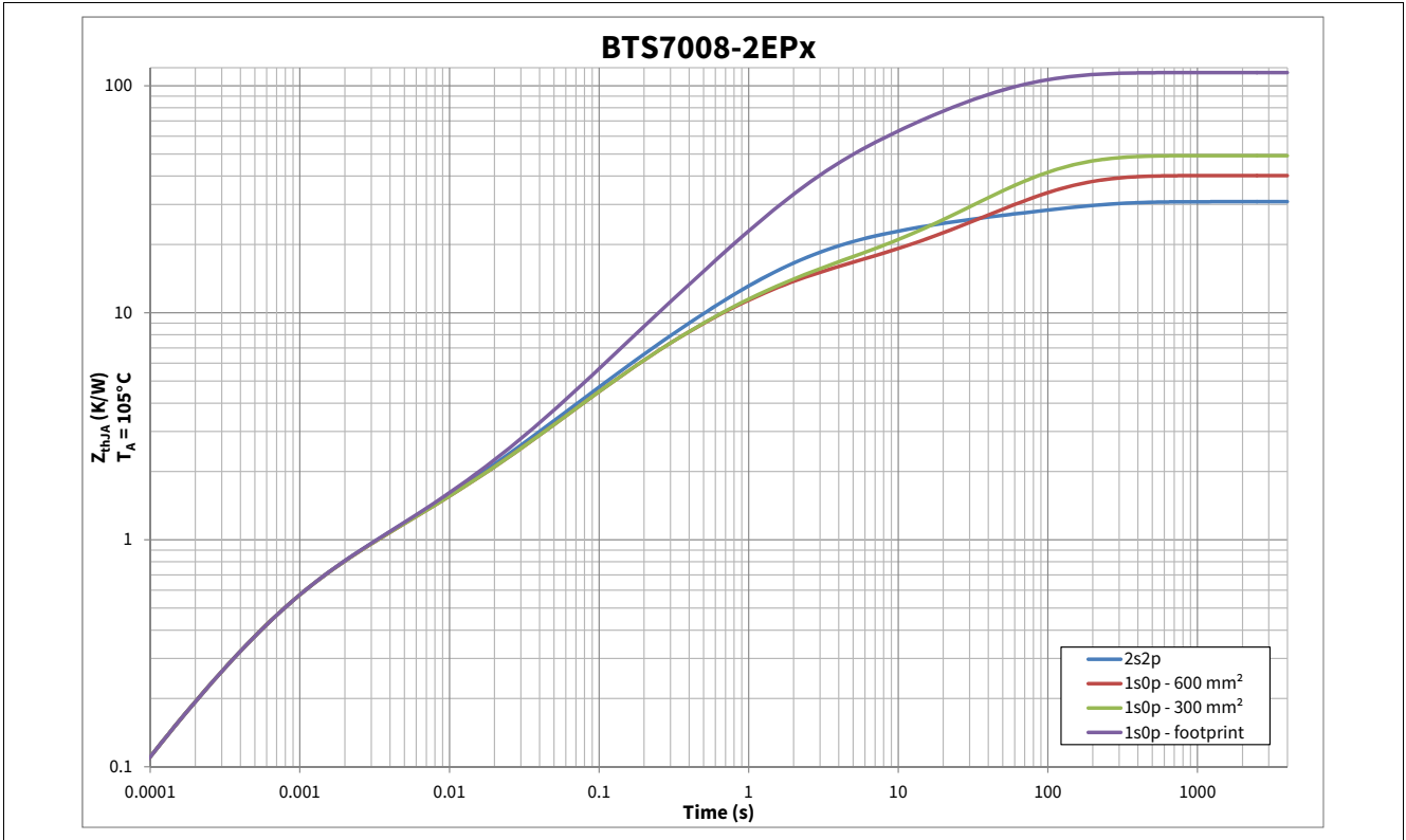
Figure 9 Typical Thermal Impedance. PCB setup according Chapter 4.4.1
