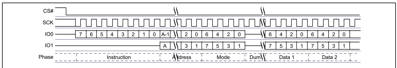
Figure 69 Dual I/O Read command sequence [33, 34]
