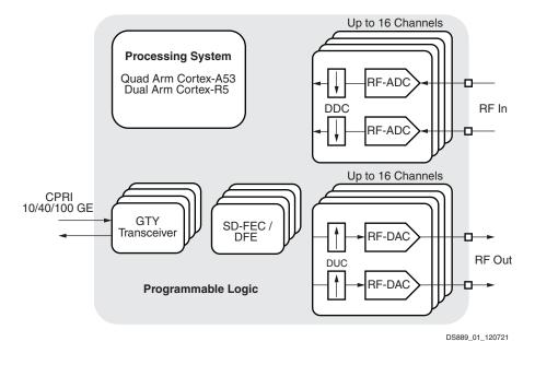
Figure 1: Zynq UltraScale+ RFSoC
