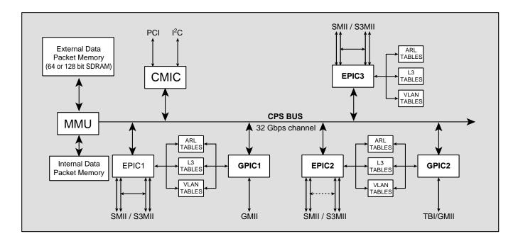
The **BCM5615**, with a forwarding rate of 6.6 Mpps, defines the next generation of performance for single-chip switching solutions. Through its advanced ContentAware<sup>TM</sup> feature set, the StrataSwitch II product family supports advanced applications and services, at wire speed, with non-blocking performance.
